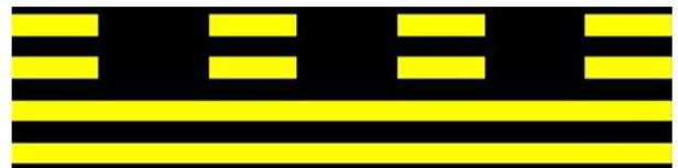
Fig 2. Runway Hold Position Marking
